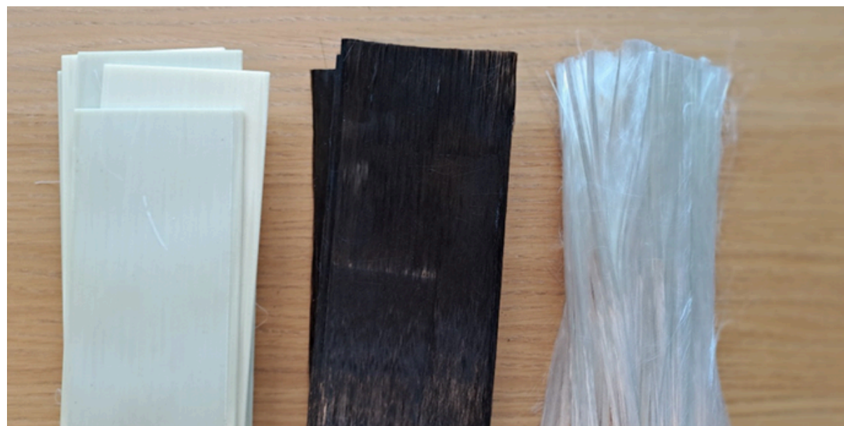
Owens Corning epoxy-based composite material used to produce wind turbine blades (LEFT), after thermolysis treatment (MIDDLE) and after calcination (RIGHT).
